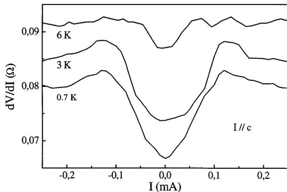
FIG. 4. Differential resistance  $dV/dI$  of a point contact between  $\text{URu}_2\text{Si}_2$  and Nb versus bias current  $I$  at various fixed temperatures given in the figure. The current was applied along the  $c$  direction.
