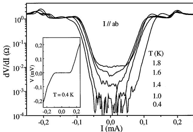
FIG. 1. Differential resistance  $dV/dI$  of a point contact between  $\text{URu}_2\text{Si}_2$  and Nb versus bias current  $I$  at various fixed temperatures given in the figure. The current was applied parallel to the  $a$ - $b$  direction. Inset: the same data at  $T \approx 0.4$  K shown in a plot of  $V$  versus  $I$ .
