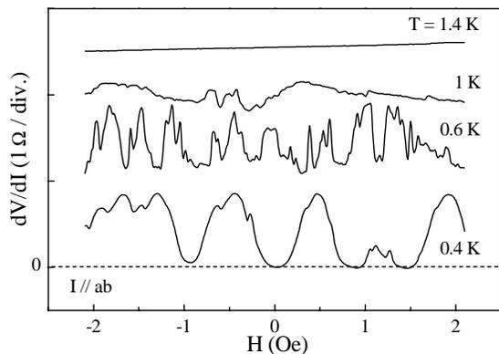
FIG. 3. Differential resistance  $dV/dI$  of a point contact between  $\text{URu}_2\text{Si}_2$  and Nb measured at various fixed temperatures given in the figure versus a magnetic field  $H$  applied perpendicular to the contact. The bias current of 0.1 mA was applied along the  $a$ - $b$  direction.
