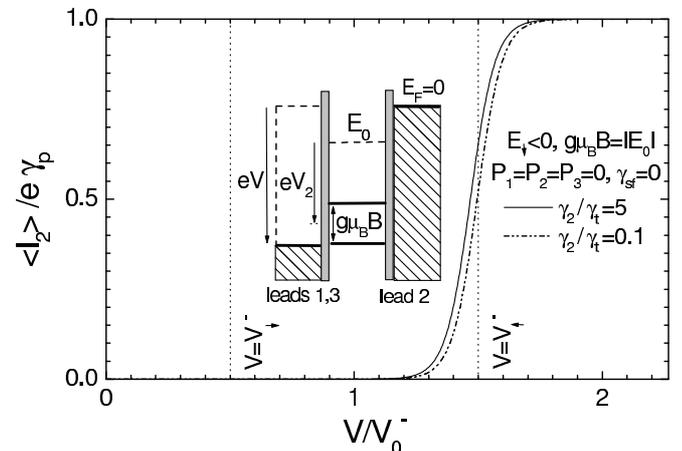
FIG. 14: Current-voltage characteristic of the circuit of Fig. 1 for  $E_0 < 0$ ,  $P_1 = P_2 = P_3 = 0$ ,  $C_1 = C_2 = C_3$ ,  $\gamma_1 = \gamma_3$ ,  $k_B T / |E_0| = 0.05$ ,  $g\mu_B B / |E_0| = 1$ , and different values of the asymmetry  $\gamma_2/\gamma_t$  between the input and the output. These curves display only one step, for  $V \simeq V_{\uparrow}^-$ . The inset shows the electrochemical potentials in the circuit.
