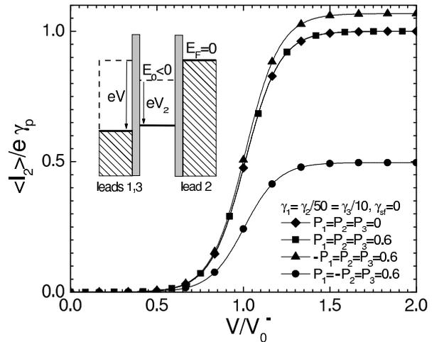
FIG. 5: Current-voltage characteristic of the circuit of Fig. 1 for  $E_0 < 0$ . The polarizations, tunnel rates, capacitances and reduced temperature  $k_B T/|E_0|$  used are the same as in Fig. 2, plotted for  $E_0 > 0$ . The results differ from the case  $E_0 > 0$  only for  $V \simeq V_0^-$ .
