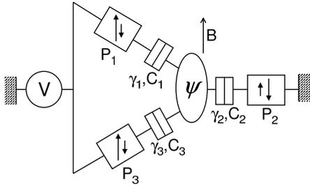
FIG. 1: Electrical diagram of a quantum dot connected to three leads  $i \in \{1, 2, 3\}$  with collinear magnetic polarizations  $P_i$ , through tunnel junctions with net tunneling rates  $\gamma_i$  and capacitances  $C_i$ . A bias voltage  $V$  is applied to leads 1 and 3; lead 2 is connected to ground. A magnetic field  $B$  collinear to the lead polarizations is applied to the dot.
