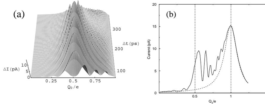
Fig. 2. – (a) Plot of pulse-induced current versus  $Q_0/e$  and  $\Delta t$ . (b) Current through the probe junction (R) versus  $Q_0/e$  with (solid) and without (dashed line) pulse of length  $\Delta t = 2T_{coh} \simeq 160$ ps. In both plots, we used the resistance ratio  $R_L/R_R = 1/1800$  which corresponds to quasiparticle tunneling rates  $\Gamma^-(2) \sim (6\text{ns})^{-1}$  and  $\Gamma^-(1) \sim (8\text{ns})^{-1}$ , i.e., like in [7].
