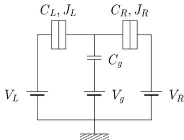
Fig. 1. – Equivalent circuit. The Cooper-pair box corresponds to the configuration  $J_L = EJ$ ,  $J_R = 0$ ,  $eV_L = 0$  and  $eV_R = -eV \simeq 2\Delta$  using the right lead as a probe gate.
