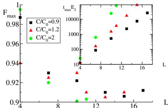
FIG. 3: Maximum value of the fidelity as a function of the length of the chain for three different values of  $C/C_0 \gtrsim 1$  and  $(2e)^2/(E_J C_0) = 10$ . Inset: time at which the maximum is reached.
