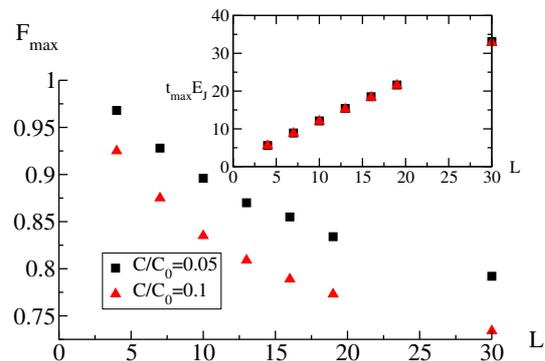
FIG. 2: Maximum value of the fidelity as a function of the length of the chain for two different values of  $C/C_0 \ll 1$  and  $(2e)^2/(E_J C_0) = 10$ . Inset: time at which the maximum is reached.
