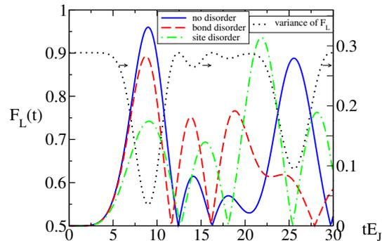
FIG. 4: Fidelity as a function of time for an array of length  $L = 7$ ,  $(2e)^2/(E_J C_0) = 10$  and  $C = 0$ , i.e. a junction capacitance much smaller than the ground capacitance. Disorder parameters: relative variance  $\Delta E_J/E_J = 0.1$  for bond disorder, absolute variance  $\Delta Q_x/2e = 0.025$  for site disorder. Dotted line (right axis): variance of the fidelity for the case without disorder.
