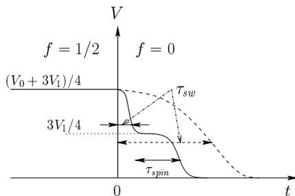
FIG. 4. Schematic representation of dc voltage  $V$  vs. time when probing the spin correlations of the DD. The flux through the SQUID loop is switched from  $f = 1/2$  to  $f = 0$  at  $t = 0$ . Solid line:  $\tau_{sw} < \tau_{spin}$ . Dashed line:  $\tau_{sw} > \tau_{spin}$ .
