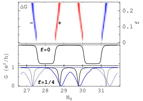
FIG. 3: (Color online) Net spin conductance  $\Delta G$  as a function of gate charge  $N_g$  and magnetic flux  $f$  in the interacting case with  $U = 0.5\text{meV}$ . Lower figures show spin-resolved conductances  $G_\pm$  for  $f = 0$  and  $1/4$ , respectively. The same plot styles and parameter values as in Fig. 2 are used. For  $f = 1/4$ , the conductances (blue lines) with a larger coupling  $t_{wr} = 0.8\text{meV}$  are also shown.
