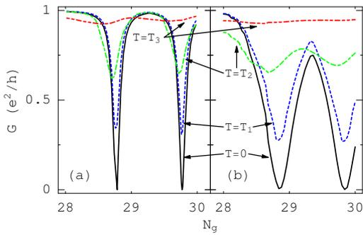
FIG. 4: (Color online) Finite-temperature conductance  $G_-$  for  $f = 1/4$ . The temperatures are given by  $k_B T_1 = 0.13\Delta(\epsilon_F)$ ,  $k_B T_2 = \Delta(\epsilon_F)$ , and  $k_B T_3 = 8.1\Delta(\epsilon_F)$ . (a)  $t_{\text{wr}} = 0.4\text{meV}$  and  $\Delta(\epsilon_F) = 0.016\text{meV}$ . (b)  $t_{\text{wr}} = 0.8\text{meV}$  and  $\Delta(\epsilon_F) = 0.064\text{meV}$ . Other parameters as in Fig. 3.
