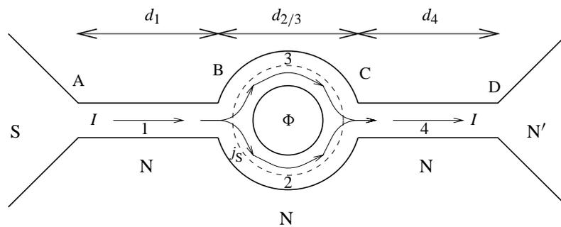
**Fig. 18.** A proximity wire containing a loop. The cross-sectional areas of the respective components are  $A_i$ .  $j^S$  is the field-induced supercurrent in the ring part.
