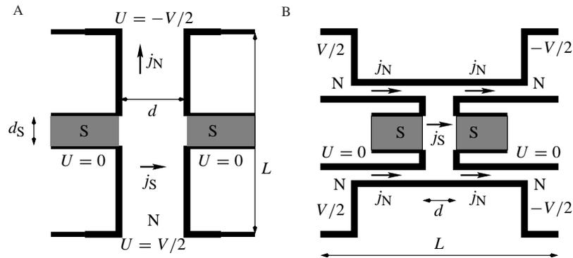
**Fig. 10.** Different realizations of the SNS transistors. The supercurrent is tuned by A, a perpendicular or B, a parallel normal current flow.
