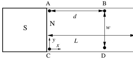
**Fig. 24.** A quasi-2D proximity film. The contacts A and B are used as voltage and C and D as current probes. An alternative setup: A and C are voltage probes, while the current flows through B and D.
